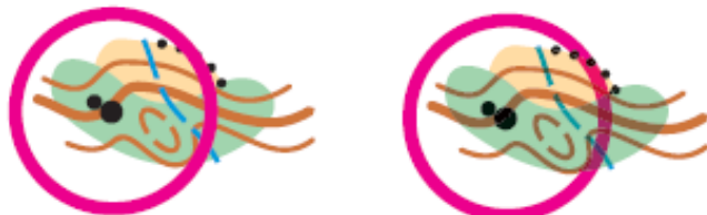
Illustration: Contours in dense vegetation printed in 4-colours. Overprinting effect in the right illustration.
